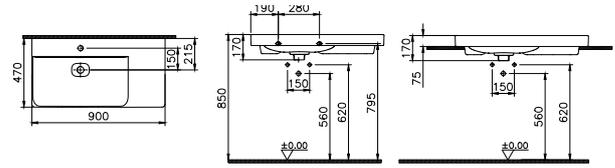
Technical drawings showing dimensions: 900mm width, 470mm depth, 75mm height, and various mounting and overflow specifications.
